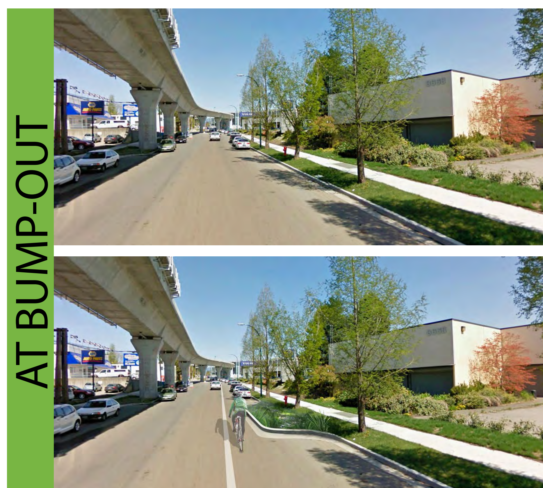
AT BUMP-OUT Ideas: Before and after view. Rain garden and bump out added at fire hydrant locations
